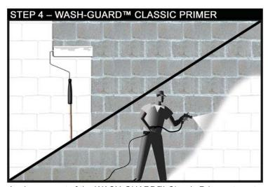
Apply one coat of the WASH-GUARD  $^{\text{TM}}$  Classic Primer at a rate of 80-100 square feet per gallon with a  $\frac{1}{2}$ "  $-\frac{3}{4}$ " nap roller ( $\frac{1}{2}$ " roller should be used on smoother surfaces and  $\frac{3}{4}$ " roller on surfaces with heavier textures) or with commercial grade airless sprayer and .015 - .025 tip.\* Allow to cure for a minimum of 4-6 hours. Use of fans in enclosed areas will speed up cure time.
