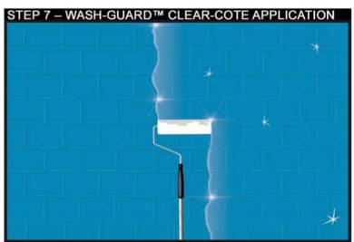
Apply WASH-GUARD™ CLEAR-COTE in two coats at a rate 350 square feet per gallon each by rolling evenly with a ½" nap quality roller cover. Back-roll to force material into any voids. Allow first coat to dry to touch before applying second coat. Be sure to roll evenly at recommended square footage rate, keeping a wet edge at all times. ANY EXCESSIVE BUILD-UP OF CLEAR-COTE WILL RESULT IN A CLOUDY FILM.
