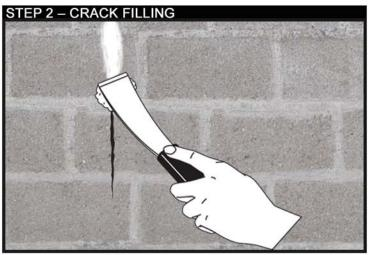
Fill cracks that are less than 1/8" with TEX·COTE® FLEX-PATCH®. Cracks larger than 1/8" must be filled with an appropriate cement patching compound. Allow patching compound to fully cure.
