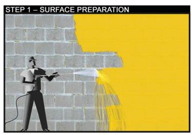
Remove all loose, flaking, or oxidized paint from the manufacturer's approved surface by water-blasting, scraping, and/ or sanding. In some cases, sand blasting may be necessary to remove any excessive build of old paints or coatings. Remove all dust and debris and allow walls to dry.
