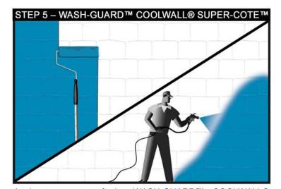
Apply two coats of the WASH-GUARD™ COOLWALL® SUPER-COTE™ at a rate of 400 square feet per gallon each coat with a ½" nap roller or with commercial grade airless sprayer and .015 - .025 tip.\* Allow to cure for a minimum of 2-4hours between coats and for a minimum of 4 hours before coating with WASH-GUARD™ CLEAR-COTE™.
