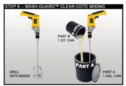
Mix WASH-GUARD™ CLEAR-COTE™ Part A and Part B components with mixing blade and drill prior to application. Begin by mixing Part A then slowly adding Part B, keeping a good vortex the entire time. Continue to mix for 2 − 3 minutes. Mixed material will have a milky appearance but will dry clear. Once mixed, material must be applied within 2 hours. Do not close the lid on unused material as pressure will build up in the can.
