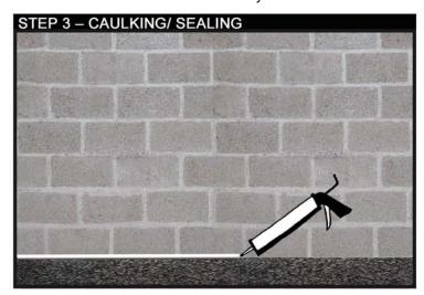
Apply a high quality acrylic caulk to the bottom edge of the wall as well as any other areas where water intrusion could occur. All surfaces must be dry prior to applying primer and moisture content should not exceed 50%, otherwise blushing or whitening of the final CLEAR-COTE may occur.
